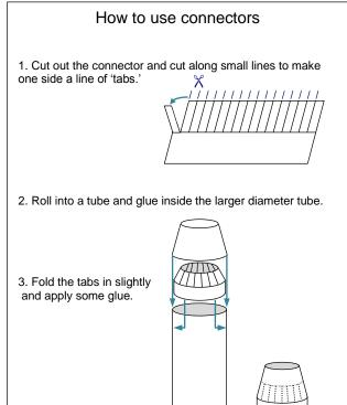
4. Attach the cone, using a small wooden or plastic rod to press the tabs to the
